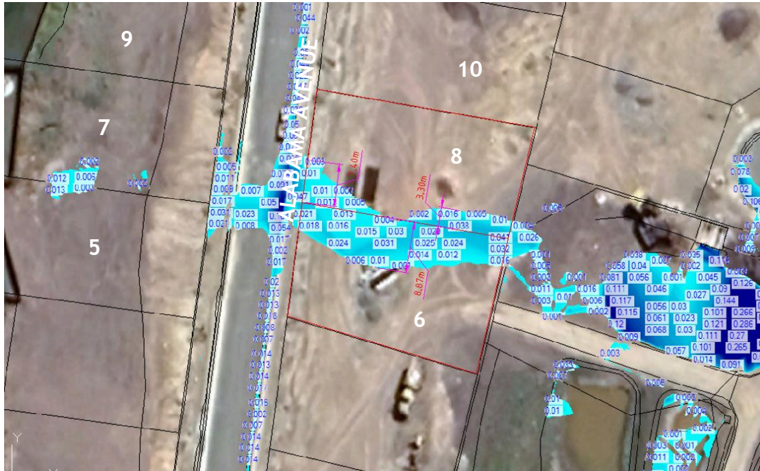
Figure 10: HEC-RAS Screenshot: Maximum Depth Along Alabama Avenue and maximum offset from the boundary of lots 6 & 8.
